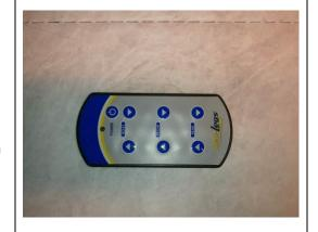
NOTE: You may find that the front of the boat rises faster than the rear. This is normal and to be expected, as the majority of the boats weight (particularly if fully rigged) is in the rear of the boat. In order to keep the boat level during ascent and descent, you may need to toggle between FRONT UP and REAR UP buttons on the remote.
